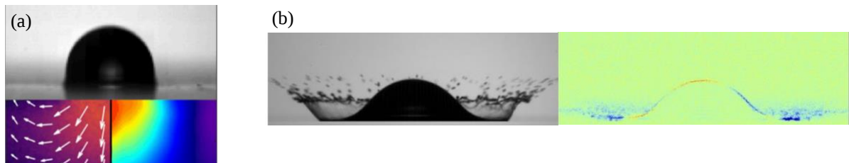
Figure 1.(a) Stress field in soft material induced by droplet impact [3] and (b) AI-based analysis of the impact [5]
