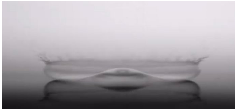
Figure 1. Example of drop impact dynamics on a superhydrophobic surface. A 3 mm-diameter water droplet impacts a CuO-based superhydrophobic surface at a velocity of 6 m/s.
